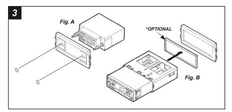
**2-SHAFT HEAD UNITS:** Slide the aftermarket head unit into the kit and secure with shaft nuts. (see Fig. A)
